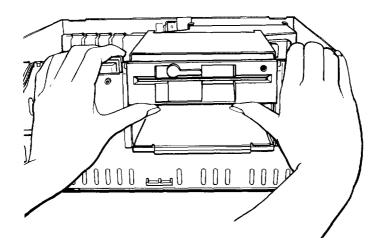
3. Raise the front of the subassembly to a slight angle, as shown below.
